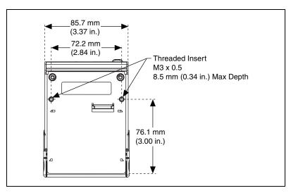
Figure 6. Module Dimensions In Millimeters (Inches)
